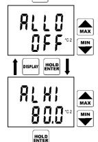
Then you are offered to set alarm of other input value (here temperature of channel 2). The procedure is the same as the above temperature limit setting. Alarm activation of each value can be disabled by setting lower alarm limit of the desired value up to its maximum. This is indicated by OFF reading at the position of numeric value. Value of upper limit of the same alarm is indifferent.
