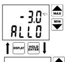
Reading ALLO indicates adjusted lower alarm limit. Set the desired value by means of the arrow keys. Press and hold the arrow key UP to make value increase fast. Press and hold the arrow key DOWN to make value decrease fast. Release the arrow key and press ENTER to confirm new limit.
