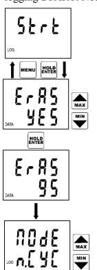
If it is needed to clear the memory before logging start, first it is necessary to select menu item logging START (symbol Strt) and confirm by pressing ENTER kev.
